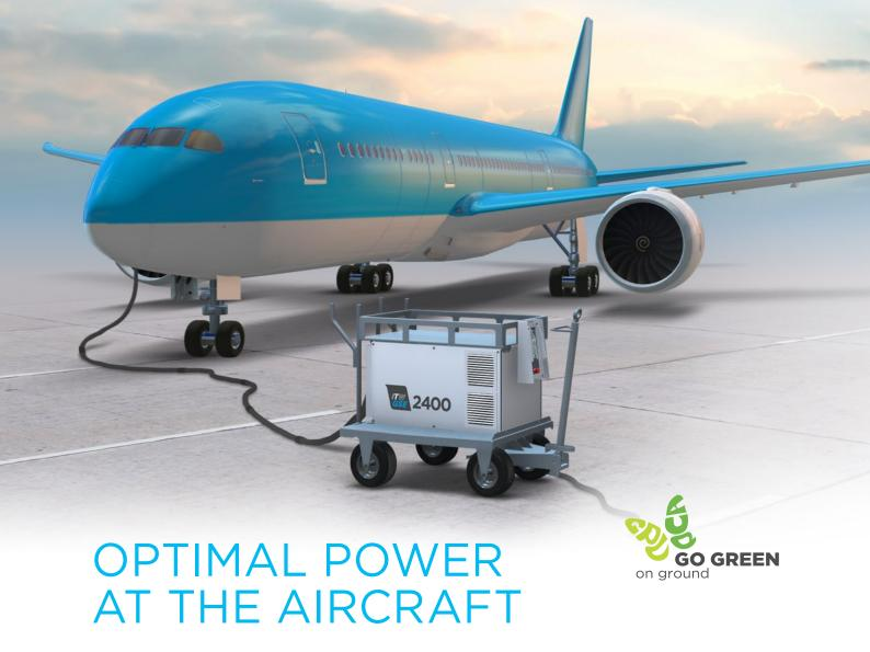
At ITW GSE, we monitor the market and are at the forefront of new aircraft requirements and market developments. This has been an objective since we introduced our first 400 Hz unit to the market. And it still is! Therefore, the ITW GSE 2400 Compact is designed to fulfil the ISO 6858 standard regarding voltage imbalance and phase displacement at the aircraft plug.
